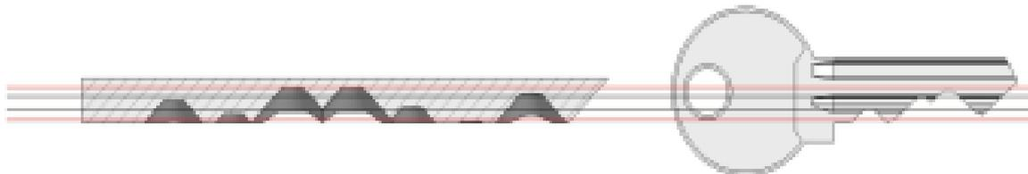
**Group 5** 1X LOCK CYLINDER WITH FULL EXTENT OF THE VARIATION FIELD FOR ANALYSIS OF THE LOCKING SYSTEM (arbitrary key cuts from the number of effective combinations)
