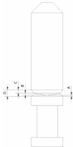
The locking system clearance (measured as well as designed) should be smaller than the declared step of the code variation. If the clearance is larger, it is assumed that the locking system was opened by the BK method or by a secondary variation.
